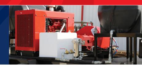
Meyer hydrostatic mobile test units are used to quickly and safely field test valves and wellhead components. Long hoses allow operator to work from a safe distance away.
